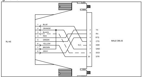
Figure 16: Modem Adapter
